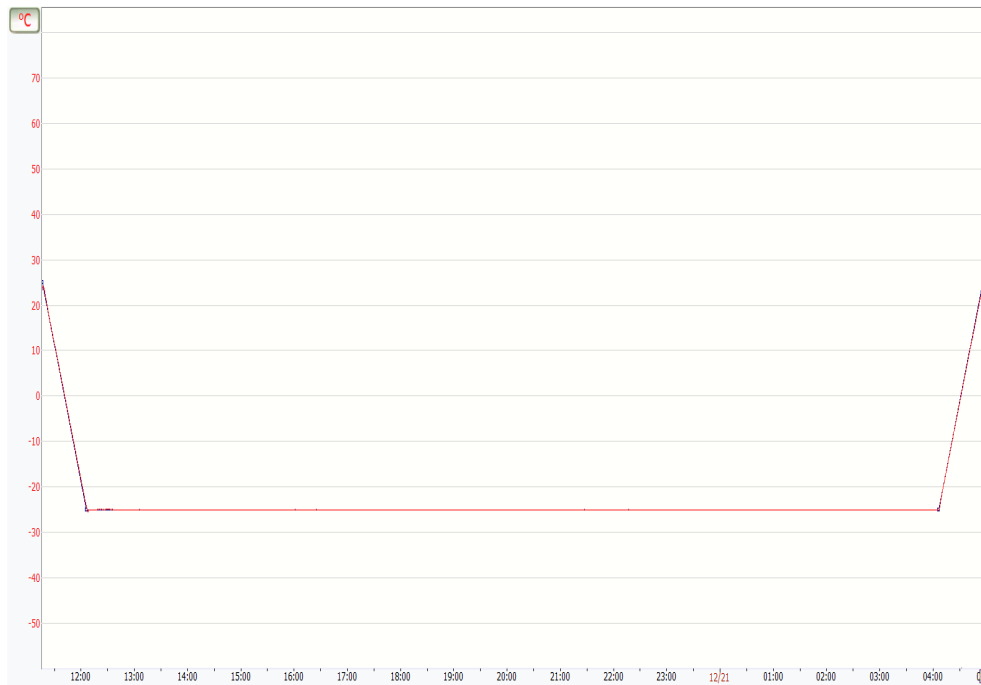
No.9 Low temperature test profile
