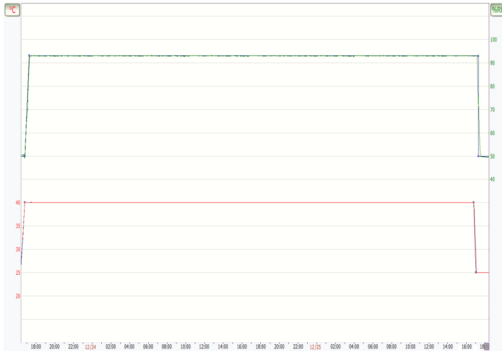
No.13 Damp heat test profile
